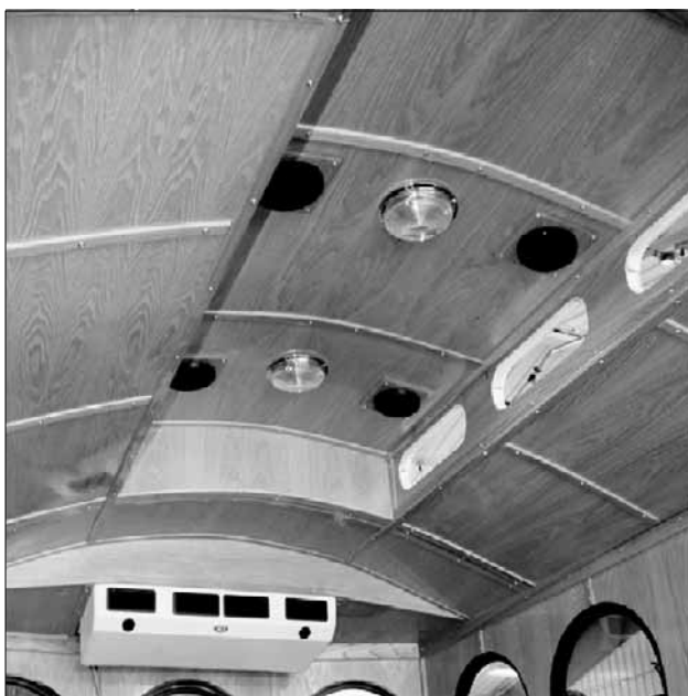
A completed ceiling in one of the trolleys
