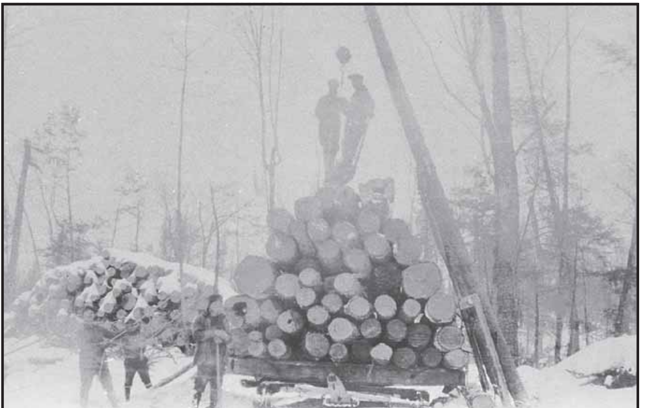
Before trucks and hydraulic loaders, logs were hauled to a railhead or to the sawmill on sleighs loaded with a-frame jammers. A team of horses was trained to pull logs up the skids seen on the left and then hold their position until the log was placed. The logs were picked up by a small hook on each end of the log, pup hooks, that were fastened to each end of a yoke that was fastened to the main line. It worked most of the time, but sometimes a hook slipped out of the log and one or both ends came tumbling down. Men were injured, and often killed when this happened, and it paid to stay on either end of the log as the two men holding the tag lines are demonstrating.
