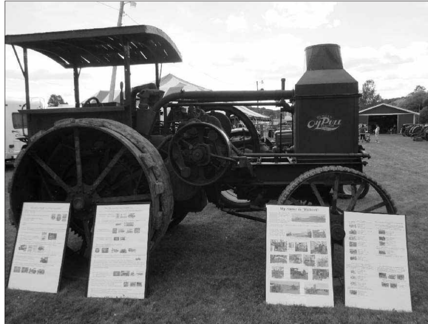
Top Left: The Ehlinger's Model T Fords. Top Right: Kids enjoy a ride around Steam Up Days. Right: A Rumely Oil Pull tractor, which ran on kerosene. Left: While not vintage, the tractor pulls were very popular.
